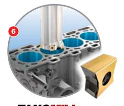
TANGENTIAL LINE Cylinder Bore Semi-Finish Boring
