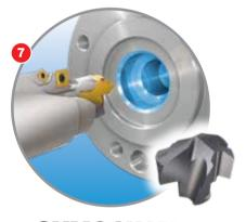
**SUMOCHAM** CHAMDRILL LINE Flywheel Mounting Flange Step Drilling and Chamfering
