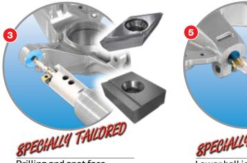
Drilling and spot face steering arm
