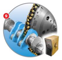
TANGENTIAL LINE Main and Pin -**External Milling**
